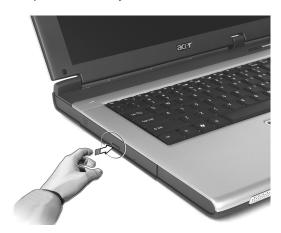
When the power is off, you can eject the drive tray using the emergency eject hole. See page 66.
